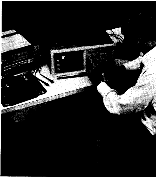
Model 1630A/D Logic Analyzer provides timing analysis, state analysis and software performance analysis in a single, benchtop instrument.
